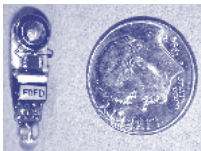
Micro-acoustic tag at 0.65 g. dry wt.; 0.39 g wet wt.; 5.5 mm x 19 mm.
