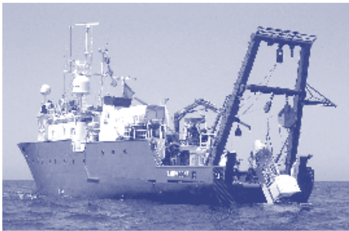
Figure 2. Deployment of LHPR off the Tarragona during cruises of P. Olivar and colleagues to study the distribution of eggs and larvae of hake, anchovy, and pilchard and their prey in the NW Mediterranean Sea.
