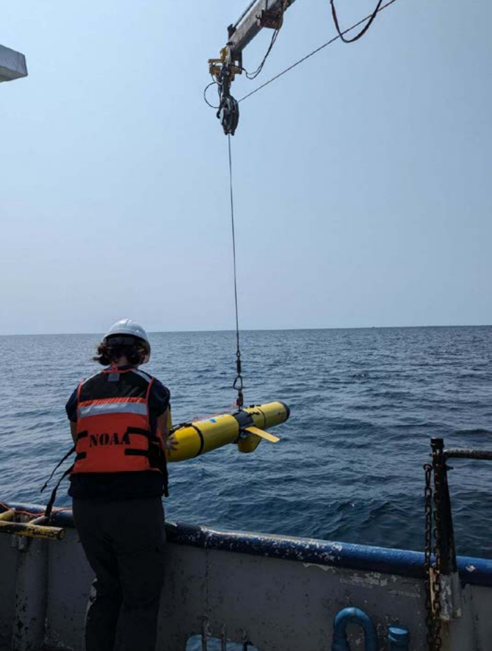
Fig. 9: Deploying the AUV glider. photo credit Paul Glyshaw
