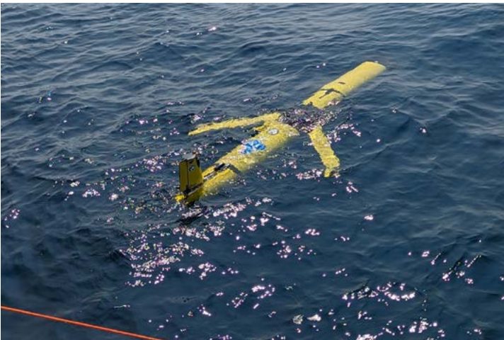
Fig. 11: AUV ready to start collecting data in Lake Michigan. photo credit Paul Glyshaw
