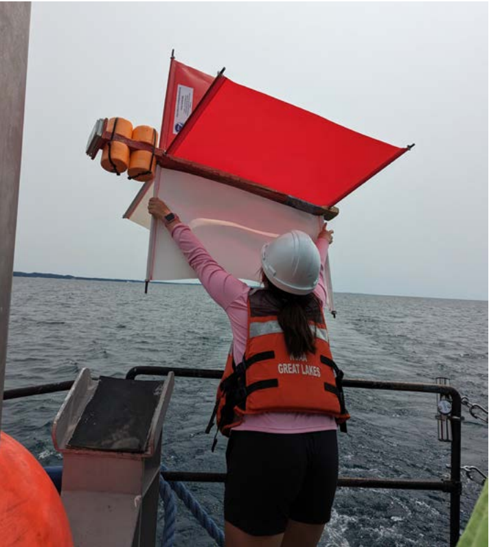
Fig. 10: Deploying tracker buoys (subsurface drifter) in Lake Michigan. photo credit Paul Glyshaw
